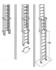
When not is use it is good practice to ensure these ladders are retracted out of reach and locked to prevent ease of access without authority.
