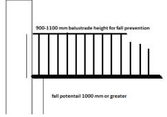
Under section F4 of the Building Code the above also applies where a there is a change in level and suitable hand rails must be provided to prevent exposure to potential falls of 1000 mm or more. *E.g.mid rail is placed at approx. 600 mm.*
