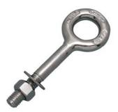
Eye bolts must be of the closed loop type as shown. Open loop types are prone to easy distortion and failure when placed under load – this means the climber can fall or equipment can be dropped causing significant risk of injury, death, and damage. When installing these make sure you have flange plates in the set up if penetrating directly through the structure as shown – these are designed to prevent the bolt pulling out through the structure when under load.
