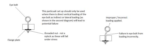
Fitting eye – bolts – must be flanged on both sides to prevent distortion and pull through of the bolt when loaded. They can be used on both wooden and steel structures. Any eye bolts installed should be stamped as load rated to 150 kg or greater.
